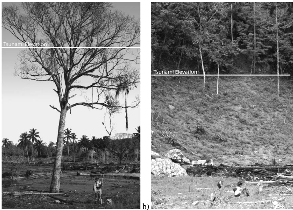
Figure 2. a) Surveying topographic profile in front of a large tree that survived the December 26, 2004 tsunami at Lhok Kruet, Sumatra. Note the branches high in the tree that were broken by the 26 December tsunami. The combination of broken branches and debris high in the tree, primarily palm fronds, indicate that the tsunami flow depth was 9.9 m at this location, which is approximately 275 m inland, b) Trimline at Jantang at 19.7 m above the sea level when the December 26, 2004 hit. Vegetation below the line was stripped by the tsunami and had begun to grow back. Note the team members examining a tsunami deposit in the foreground. Photographs taken by Bruce Jaffe.
